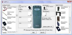
connected. Or, if your sensor is not auto-ID, you can simply drag the sensor to the appropriate channel.
