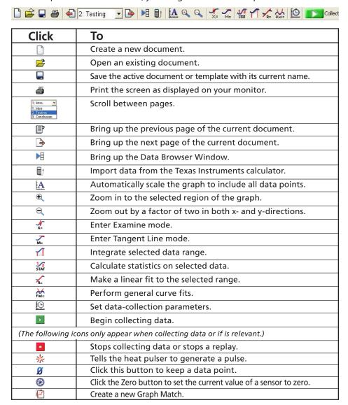
**Menu bar** Logger *Pro* has a menu bar across the top of the main window. Use the menu bar to access all of the software's features.
